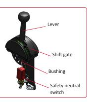
environmental conditions while providing optimal UV protection. The result is a shifter that outperforms virtually all other OEM shifters. In addition, the Forward, Neutral, and Reverse are illuminated by an LED light for clear and easy visibility. A Cole-Hersee<sup>®</sup> electric safety neutral switch increases safe operation of the shifter.
